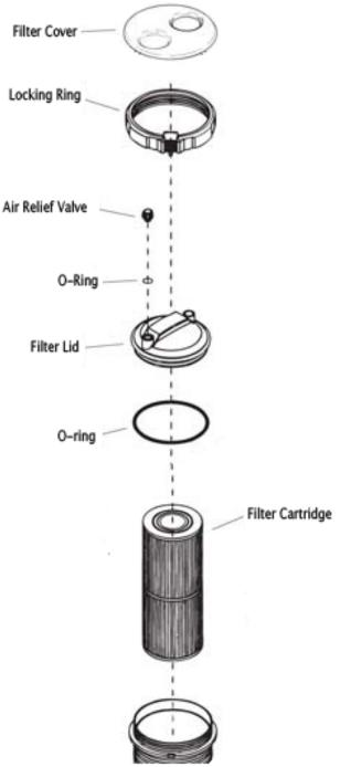
• Reinstall filter and lid and turn power ON to the spa. Tighten air relief valve once any trapped air has been bleed off.
